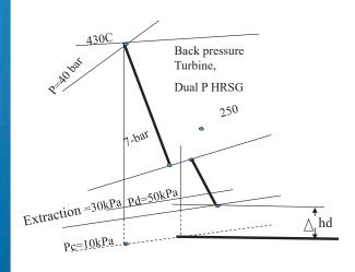
If the back pressure is high in the order of in excess of 5 bar a low pressure turbine can be retrofitted. But design for MSF and MED is based on low pressure such as 2 to 3 bar back pressure it is highly unlikely to get a low pressure turbine.
